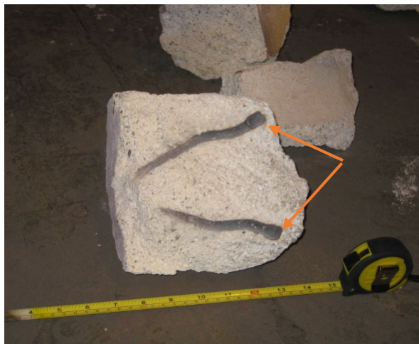
Fig. 3. Tear out of castable installation showing the imprint of an anchor with caps
