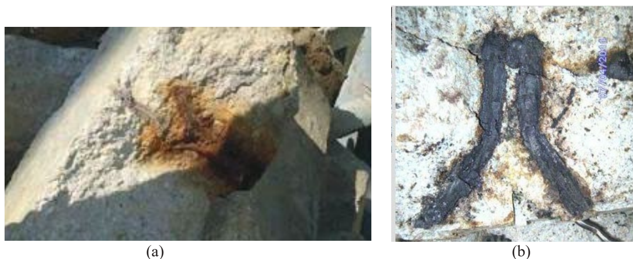
Fig. 8. Oxidation: (a) effect of alternate fuels on anchor integrity: cast walls in the riser duct of a cement kiln 25 , (b) highly corroded anchor (Cooler Bull Nose Section) 22
