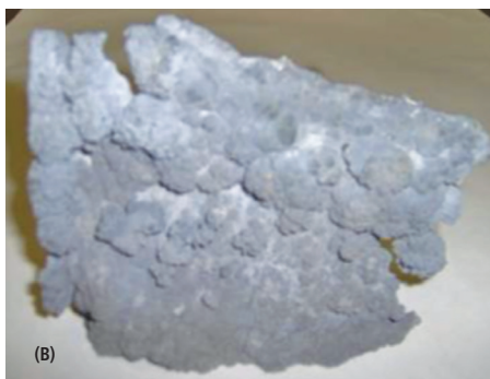
Fig 4. Corundum: (A) build up on refractory sidewall, (B) piece removed from a surface [5]
