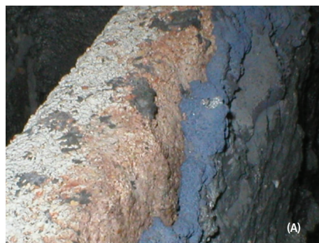
Fig 4. Corundum: (A) build up on refractory sidewall, (B) piece removed from a surface [5]
