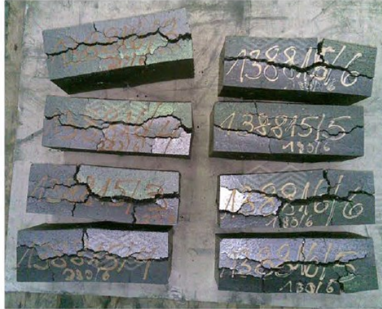
Tempered MgO-C bricks produced with \text{Al}_4\text{C}_3 -containing secondary raw materials*8
